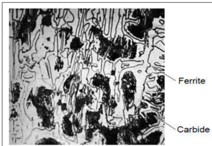
Figure 2.5 Microstructure of white cast iron
