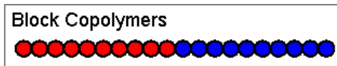
Fig.3.8. Schematic representations of Block copolymer
