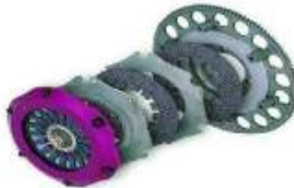
Fig: Exploded View Of Multi-Plate Clutch
