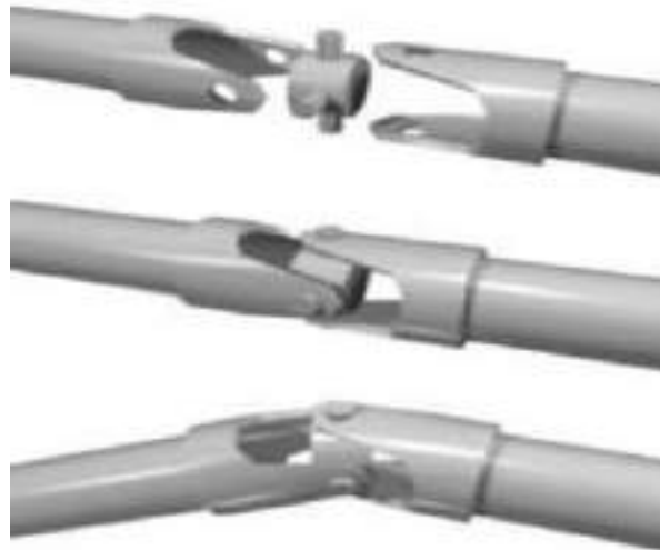
Fig: Components and assembly of U-Joint
